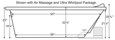
IMPORTANT: Air baths and tubs with a pre-leveled foam base or frame system add 2-3" to overall tub height.
